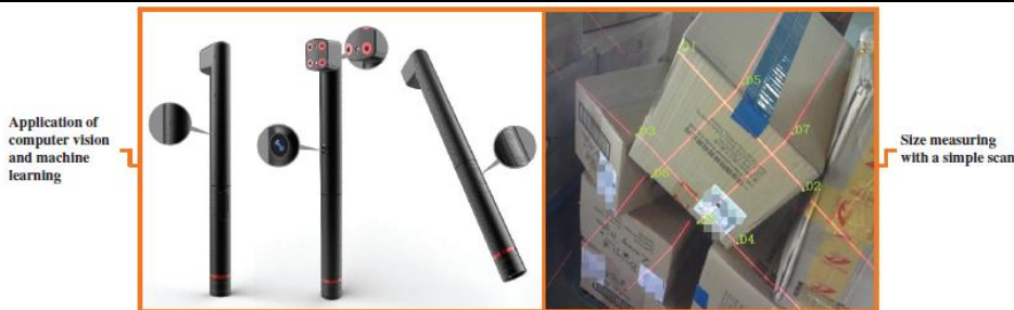
Figure 32: Fleet Size Scanning with the Application of Computer Vision and Machine Learning
